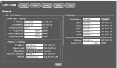
IP addresses are assigned to respective USF-105S modules installed. Refer to USF-105S operation manual Sec.10 "USF-105S Web GUI" for details on setting IP addresses.
